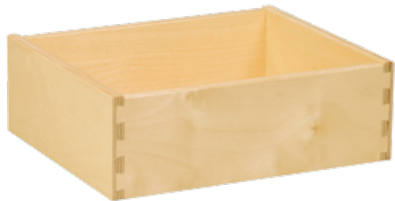
Dovetail Drawer Box (661) 1/2" Sides, 3/8" Bottom Prefinished 9-Ply Birch
